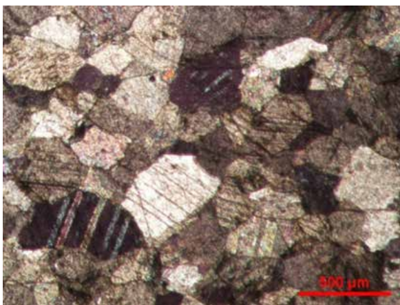
FIG. 7. Detail of the texture, showing the GBS (straight to curved) and the MFS ( \leq 0.4 mm). Photomicrograph in crossed polarized light.
