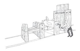
Fig. 2. Fulling Mill from Toledo. Source: Caro Baroja, 1966, p. 467
