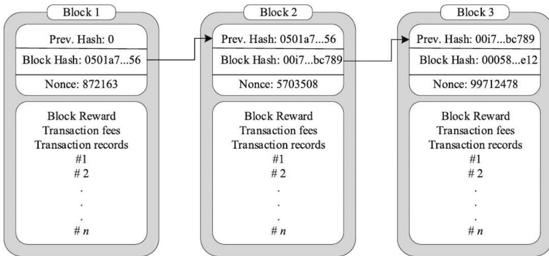
Figure. 1 Structure of bitcoin blockchain for three the blocks.
