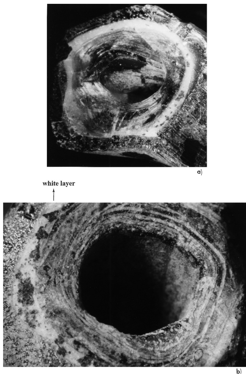
FIG. 17. Multi glass layers structure in the endpoint of beads – Set II. a) Endpoint of bead n.º 1. b) Endpoint of bead n.º 2.
