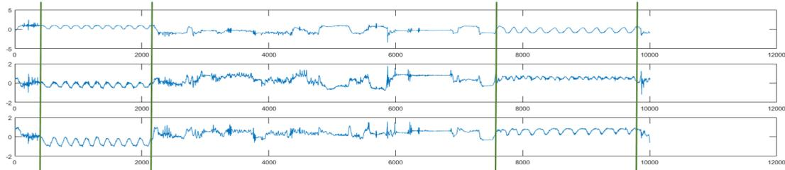
Figure 3: 3 acceleration signals ( $x,y,z$ ) corresponding to two different gym exercises (separated between vertical lines) and null-data between the exercises.
