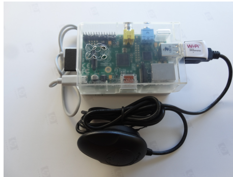
Figure 8: Raspberry Pi Broadcom BCM2835 SoC full HD, 700MHz Low Power ARM1176JZ-F, 512MB SDRAM, 256MB SD with Raspbian, Wi-Pi Wireless Adapter (802.11n up to 150Mbps), GPS receiver NL-302U (baud rate: 4800 bauds) and a dual output 5000mAh battery.
