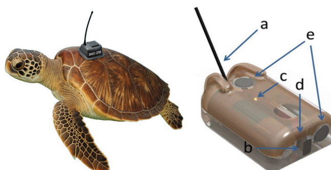
Figure 3. SPOT-375B sensor specifications: (a) Argos transmission antenna, (b) communication port, (c) LED status indicator, (d) magnetic activation switch, and (e) wet/dry immersion sensors
