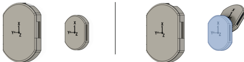
Figure 7. Representation of the initialisation process of the two sensors. Left: no transformation; right: rotation and lateral movement transformation
