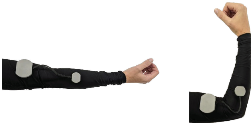
Figure 4. Photographs of the wearable device worn by the user. Left: extension of the elbow junction, close to 0 degrees angle, calibration position; right: flexion at an approximation of 90 degrees
