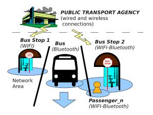
Figure 3: Structure of the Smart Transport System.
