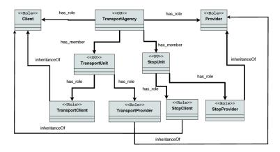
Figure 7: Structural model of TransportAgency.
