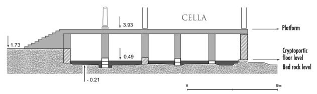
Fig. 3. Cross-section of the Augustan cryptoportico of Conimbriga, with the hypothetical reconstruction of the staircase giving access to the platform and of the level at which it is found.
